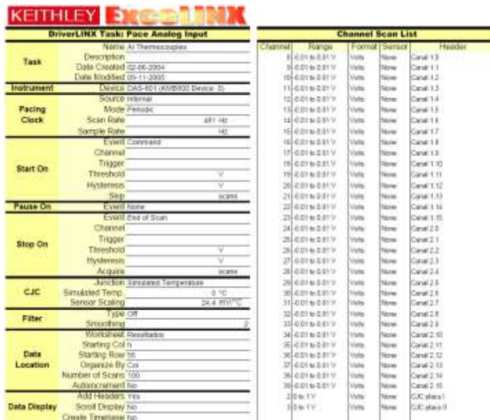
Figure V-7 – Data acquisition control panel – thermocouples and CJC sensors.
