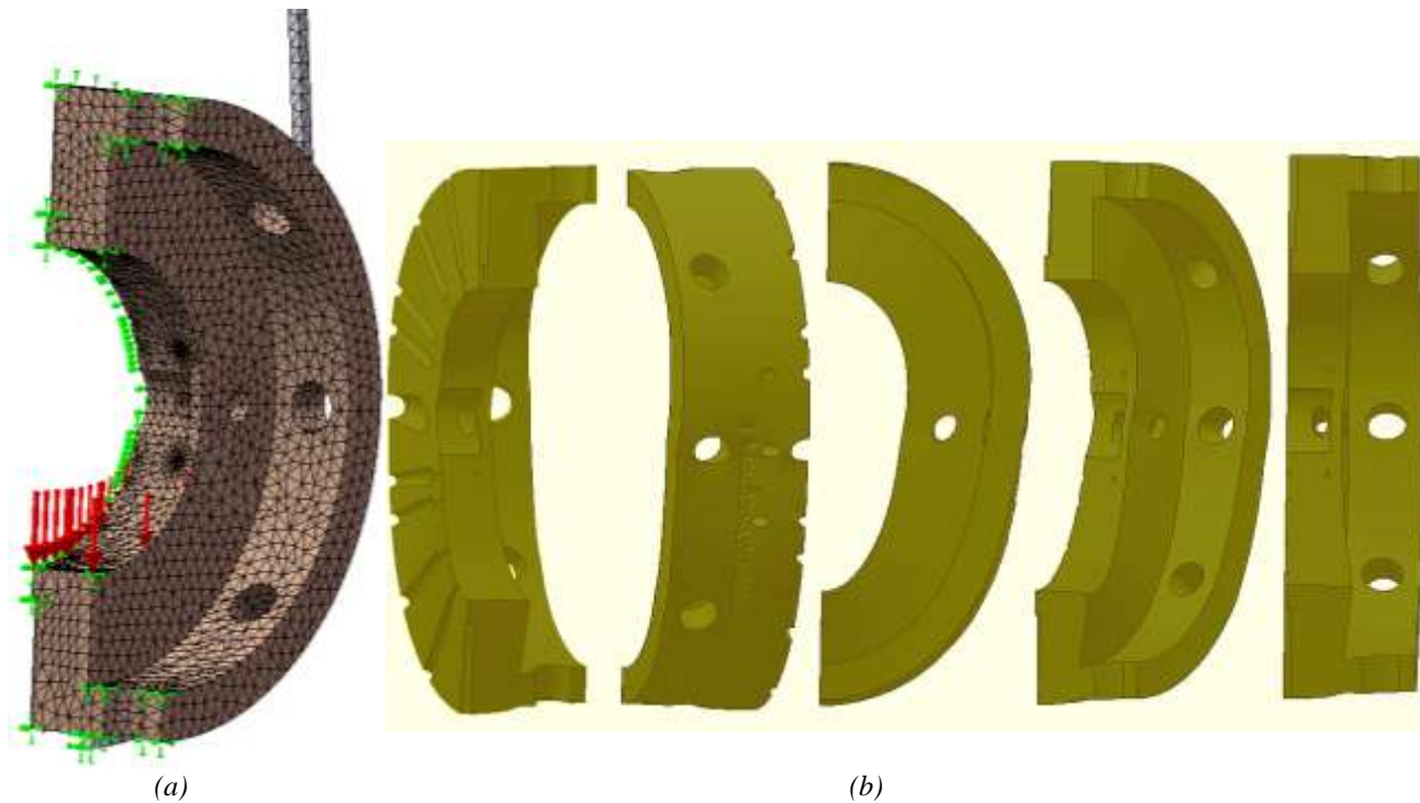
Figure V-17 – Finite Element simulation of the elastic displacements suffered by the bush (B3) and the cable subjected to a 5kN load, (a) meshing and boundary conditions ; (b) elastic deformation displacements (magnified 1500 times). Note: Taking into account symmetry, simulation was made only with \frac{1}{4} of the bearing.
