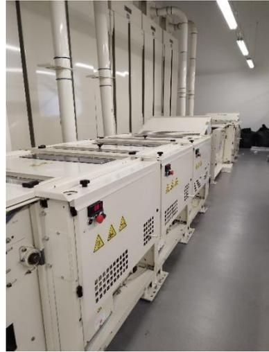
Figura 21-Desfibrador (Defibrator machine).
