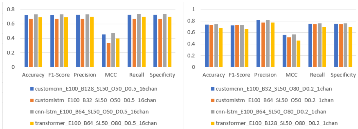
Figure 17: Comparative analysis of EEG channels: Hold-Out (1st iteration) with CAR datasets at different speeds (1.6 km/h and 2.5 km/h) using 16 (Left) and 1 (Right) EEG channels.
