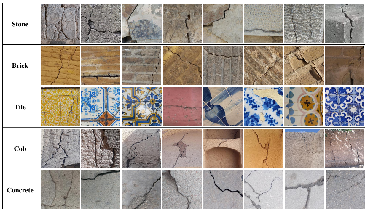
Figure 2: Sample images from five datasets showcasing various materials with cracks (stone, brick, tile, cob, and concrete)
