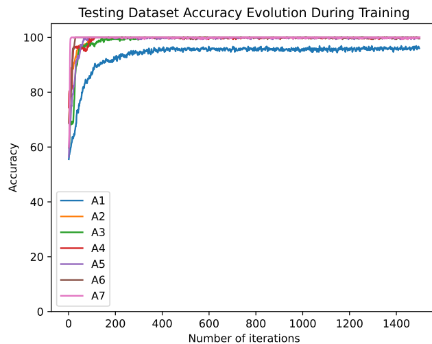
Figure 57: Comparison of Quantum Circuits with Different Numbers of Ansatz Layers (A1-A7) and Two Encode Layers (Smoothed Curves).
