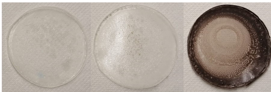
Figure 58: Films deposited on Petri dishes: ionic liquid and PVA in a ratio of 3:1 (left) with 5 or 10 mM of \text{AgNO}_3 (center and right, respectively).
