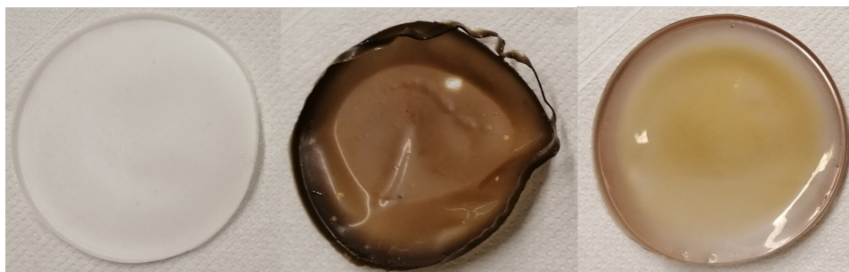
Figure 55: Films formed on Petri dishes: ionic liquid and PVA in a ratio of 0.8:1 (left), with 5 or 10 mM of \text{AgNO}_3 (center and right, respectively).
