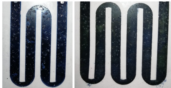
Figure 53: Photographs of the damaged films after immersion in \text{NaBH}_4 .
