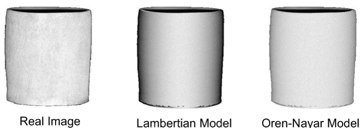
Figure 22: Comparison between a real photograph, a render using the Lambertian model, and using the Oren-Nayar model. Source: https://www.cs.columbia.edu/CAVE//projects/oren/
