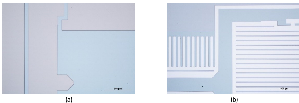
Figure 5-15 – OM images of BS double lithography process to create multilevel mask without grayscale lithography.
