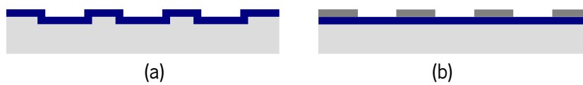
Figure 4-28 – Binary reflective DOE by (a) substrate with reflective coating followed by different material reliefs or (b) substrate etching followed by reflective coating.
