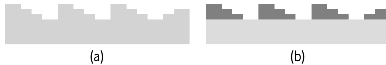
Figure 4-27 – Multilevel DOE by (a) different material reliefs or (b) substrate etching.
