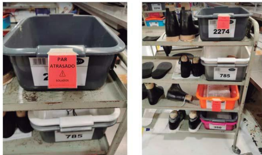
Figure 6. Application of the Visual Management as solution for late pairs on the shop floor (Par Atrasado = Late Pair).
