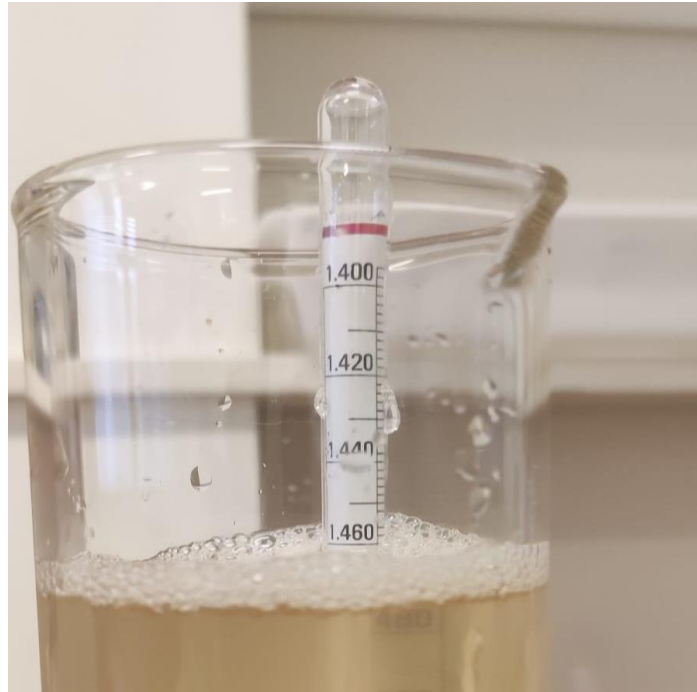
Figure 30 – Saline solution with density >1.4g/cm 3
