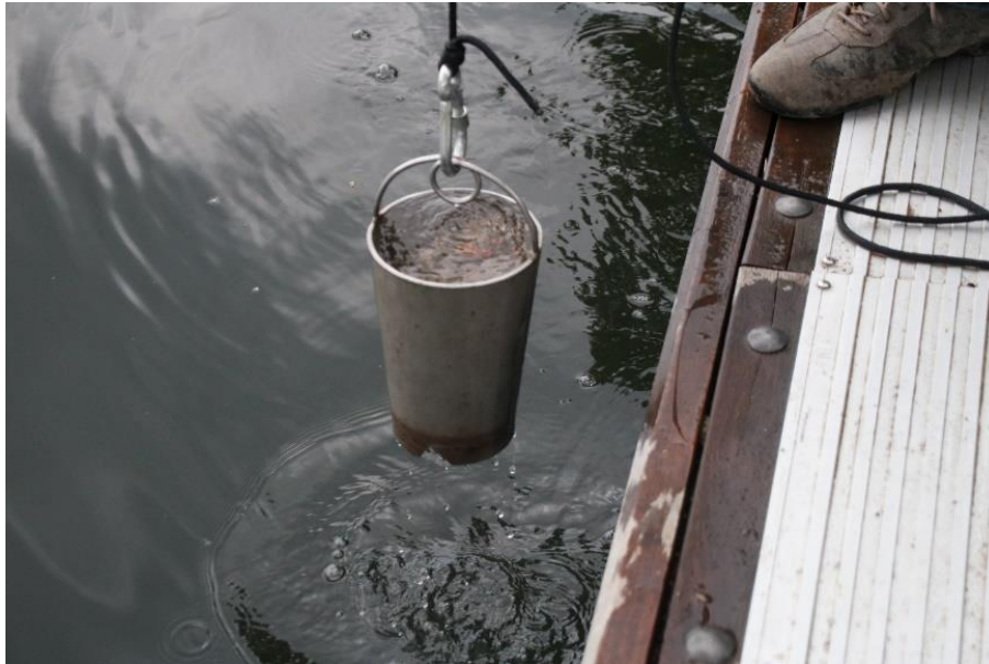
Figure 24 - Sampler: a stainless-steel bucket ~ (15cm diameter x 30cm height).
