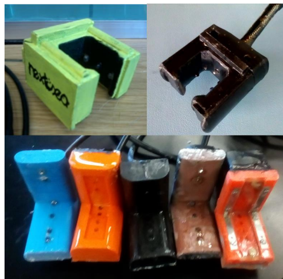
Figure 19. The top images showcase U-shape SPM Sensors and the bottom image displays a set of L-shape SPM Sensors.
