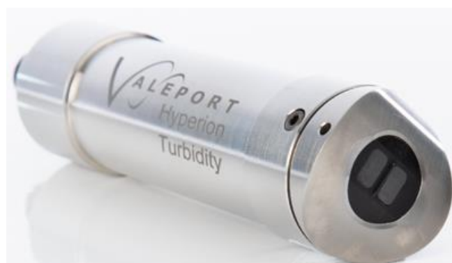
Figure 10. Valeport Hyperion-T. Standalone commercial turbidity sensor that uses nephelometry technology for lower turbidity levels (0 to 1000 NTU) with a minimum detection level of 0.03NTU, and backscattering technique for higher values (1000 to 6000 NTU). The sensor is built in titanium housing and can be submerged up to 6000 m.
