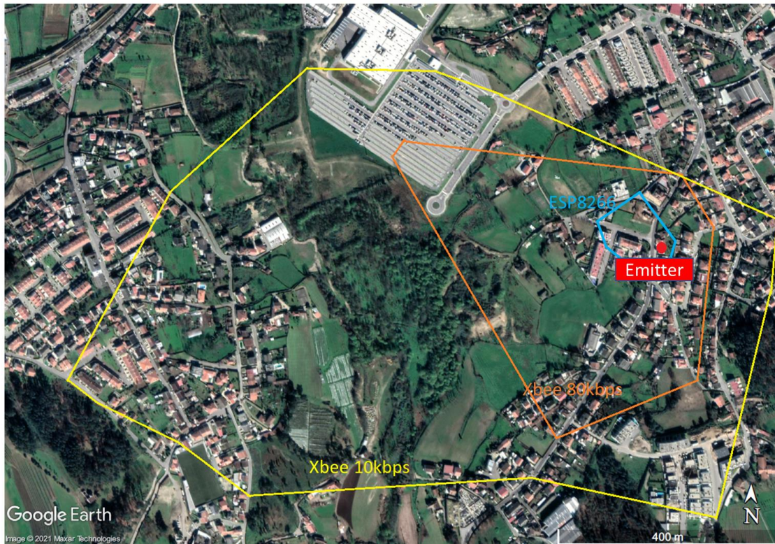
Figure 70. Results of a communication range test in an urban area using a Digi Xbee mesh with transmission rates of 10 kbps (yellow line) and 80 kbps (orange line), and an ESP8266 network (blue line). The emitting module was placed in a location with a clear line of sight to the west.
