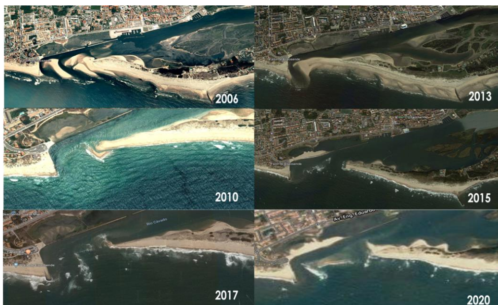
Figure 72. Satellite photographs that show the changes in the geomorphology of the estuary of Cávado River during the last decades. The inlet of the river mouth has been suffering several changes and shallow formations that are a constant problem for the navigation of the channel.
