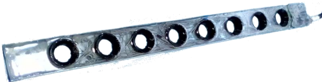
Figure 28. Image of the TVP Sensor. The instrument comprises 8 monitoring nodes with the backscatter and transmitted light channels along a 645 mm bar and it is intended to be placed vertically in the water column to measure the vertical turbidity profile.
