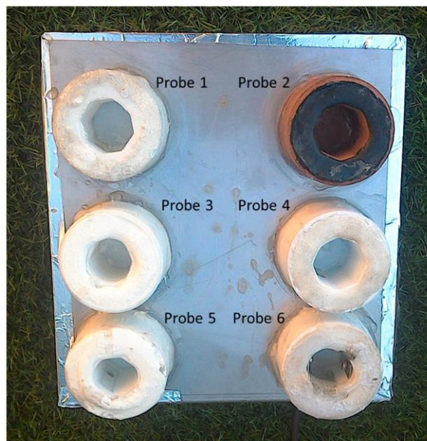
Figure 67. Anti-biofouling techniques probes. Probe 1: ABS material; Probe 2: PLA with copper filament; Probe 3: PDMS coating; Probe 4: PLA material; Probe 5: epoxy coating; Probe 6: chlorine production.
