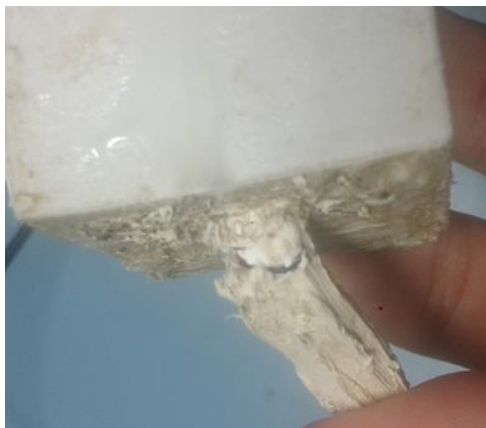
Supplementary Material VI 3. Photographs of the prototype I of the SeT Sensor after and at the end of the experiment. The right image shows a photograph of the damaged cantilever. The left image shows an underwater photograph of the sensor at the recovery day.
