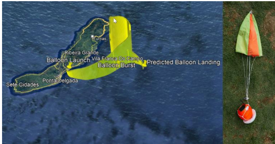
Figure 111. The left image presents the flight simulation of the HAB. The right image presents a photograph of the atmospheric probe with a parachute before the launch.
