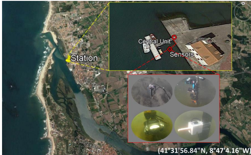
Figure 73. Installation of the monitoring station in the estuary of Cávado (41°31'56.84" N, 8°47'4.16" W). The first inset image shows the position of the central unit (outside the water) and the position of the sensors (underwater). The second inset image shows underwater photographs of some of the sensors installed: the SDE Sensor at the top left, a set of SPM Sensors at the top right, the acoustic ToF current meter at the bottom left, and the second prototype of the SeT sensor at the bottom right.
