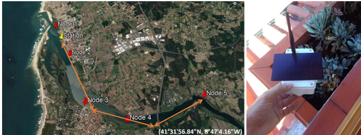
Figure 123. The image at left shows the location of the monitoring station, the 5 new locations of the XBee nodes and in orange arrows the test of XBee network coverage. The image at right shows the data logger housing with an IPV6 waterproof housing, solar panel and RF antenna.
