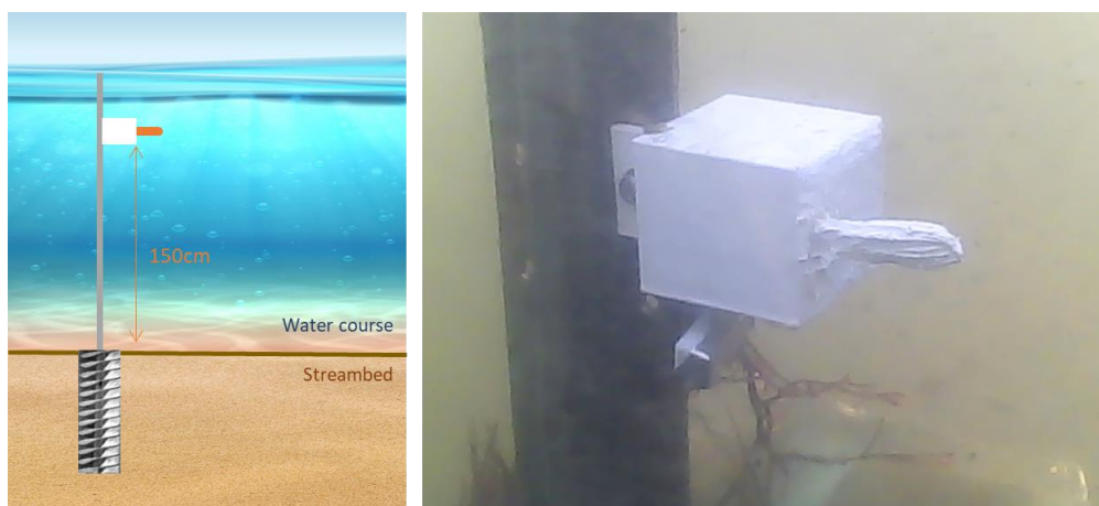
Supplementary Material VI 1. Illustration and underwater photograph of the installation setup of the prototype I of the SeT sensor. The right image shows the sensor during the installation.
