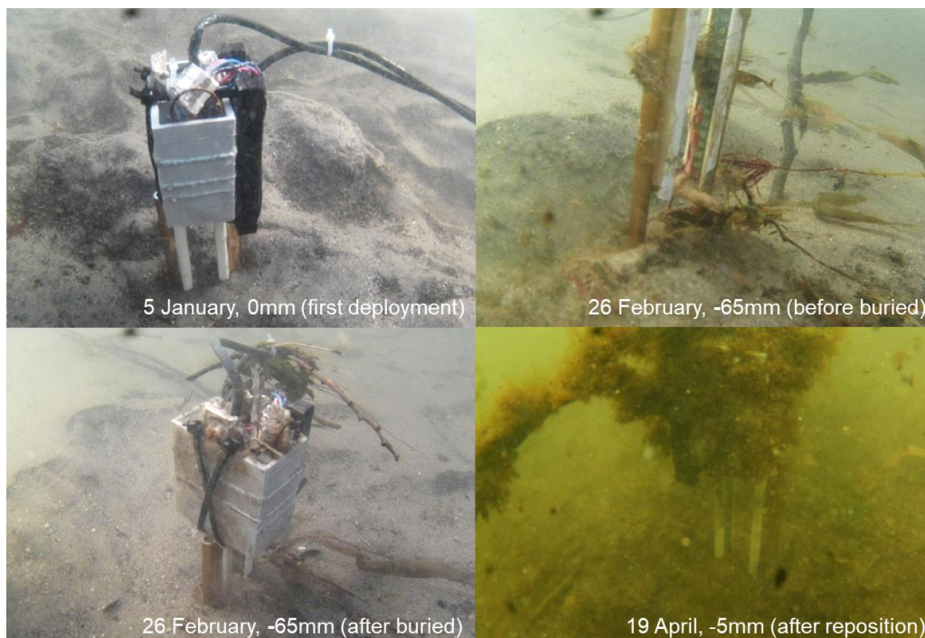
Figure 89. Underwater photographs of the SDE sensor at different times of the field experiment. The top-left image shows the moment when the sensor was deployed, with its measure corresponding to 0 mm. The top right image shows the sensor with all 32 optical channels completely uncovered (26 th of February, measure corresponding to -65 mm). The bottom-left image, also on the 26 th of February, shows the sensor buried again in the streambed (only the vertical position changed). The bottom-right image shows the repositioning of the sensor, on the 19 th of April, after the sensor was buried in sand and algae.
