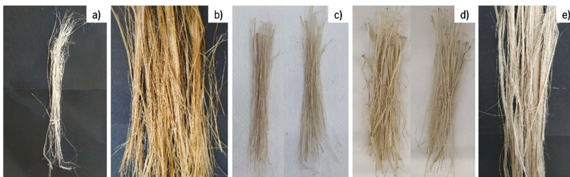
Fig. 3. Fibers obtained from the different extraction procedures: a) hand scraping only; b) NaOH; c) water retting at room temperature (7 and 21 days, respectively); d) water retting at 35 °C (14 and 28 days, respectively) and e) boiling water.
