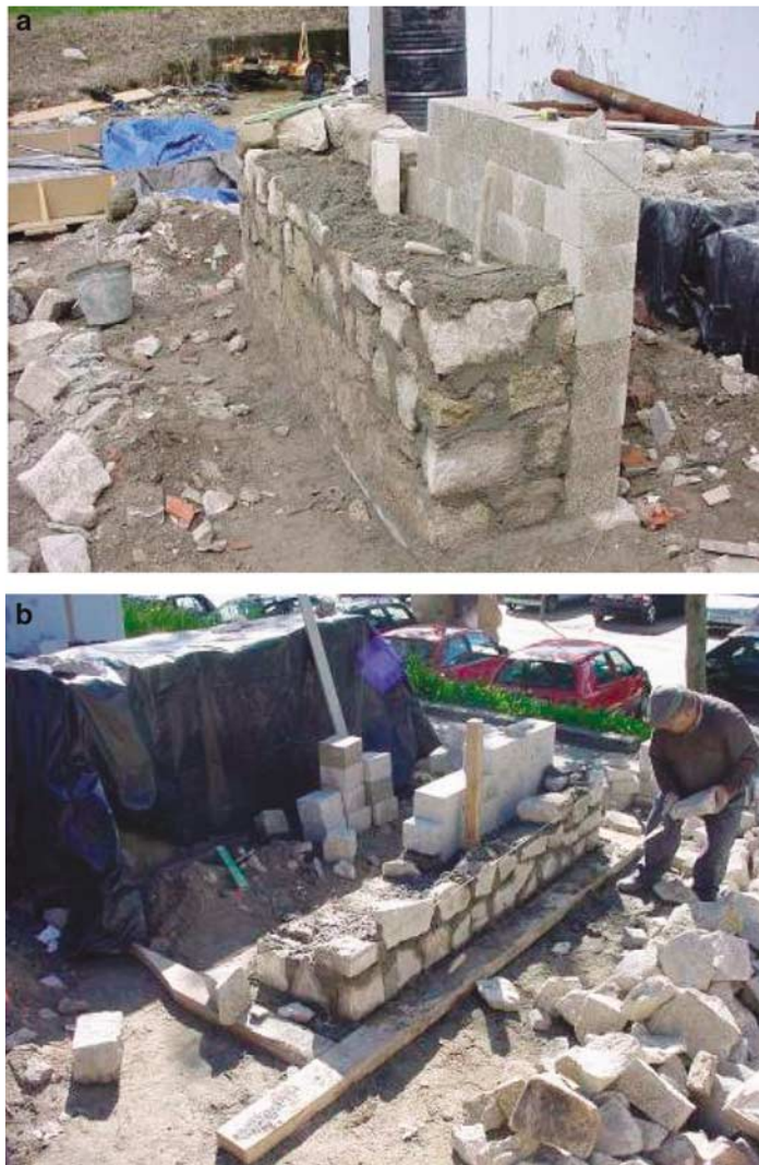
Figure 13: View of the embedded objects: (a) polystyrene prism and (b) wood beam
