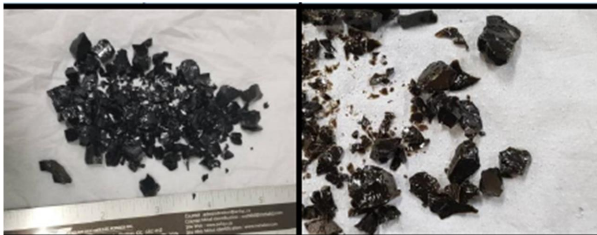
(Figura 5.39) Figure 7. Glass formed from GlassRock™ methodology demonstrates the possibility of As and Sb recovery and its use as an industrial product.
