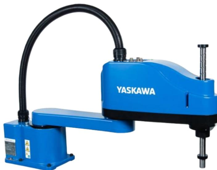
Figura 6: Robôs SCARA (Robô Scara , 2023)
