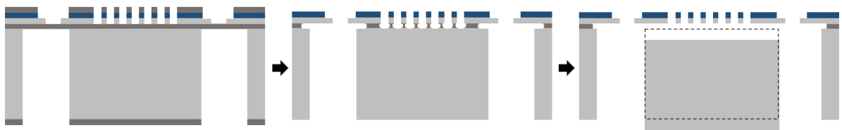
Figure 5.19: Structure release, silicon oxide etch.
