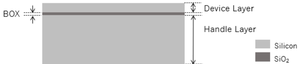
Figure 5.1: SOI Wafer cross-section.
