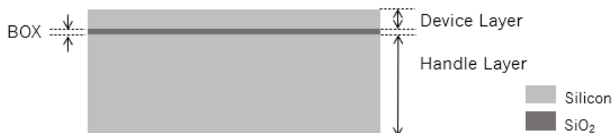
Figure 4.2: Cross section of the SOI wafer.
