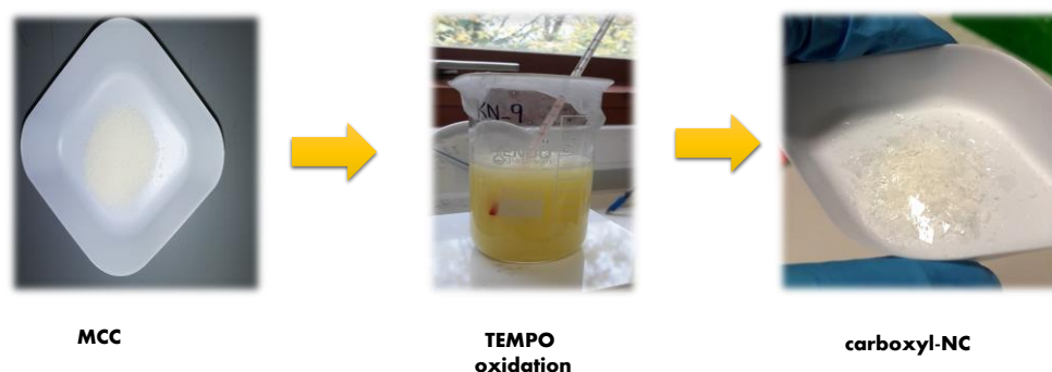
Figure 3-1. Synthesis of the carboxyl-NC by TEMPO oxidation of MCC.
