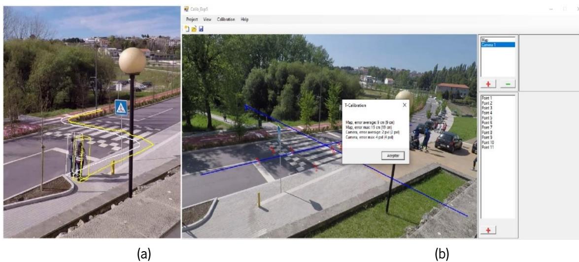
Figure 29. Example of pilot experiment (a) tracking using T_Analyst and (b) calibration using T_Calibration.
