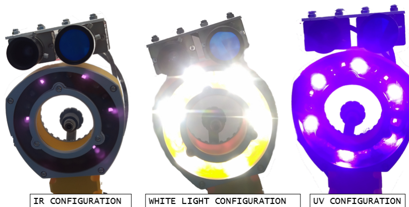
Figure 4.6: EFFI-RING different light modes with cameras attached
