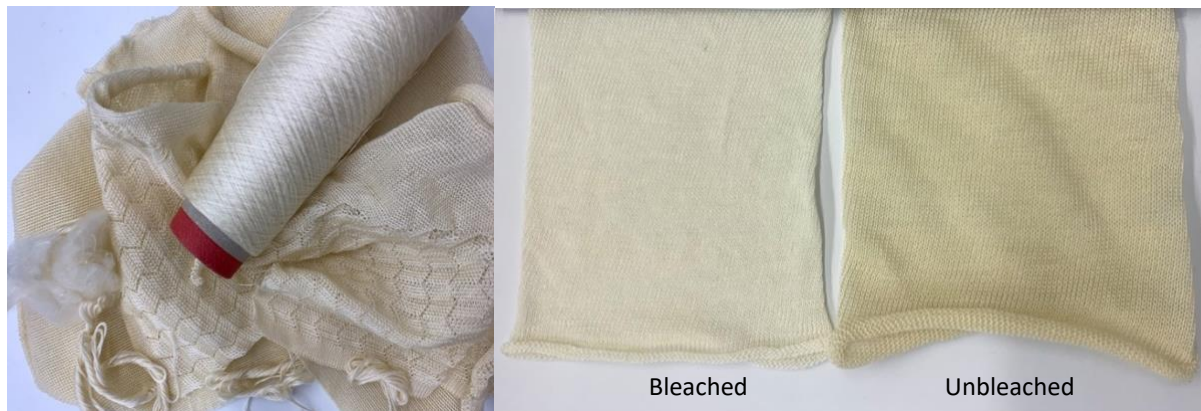
Figure 7.8. On the left: picture of fibres, yarn and knitted BC; on the right: unbleached vs bleached knitted BC samples
