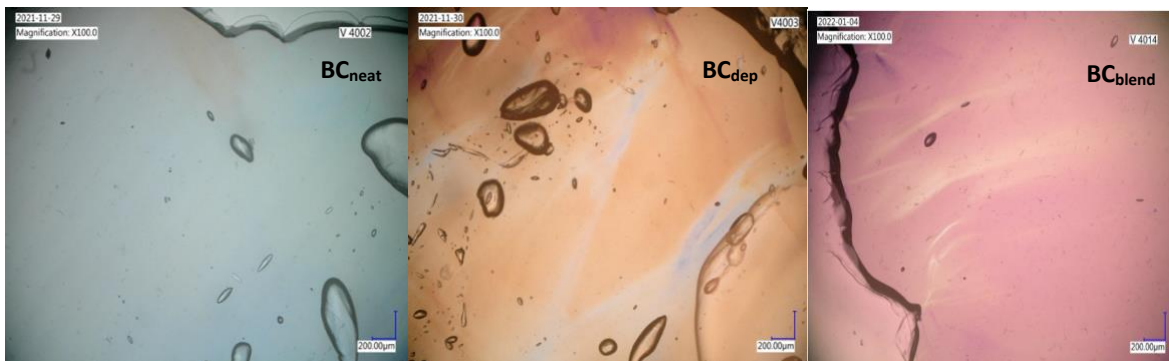
Figure 6.3. Microscopic images (polarized light) of the different BC dopes (scale division 200 \mu\text{m} )
