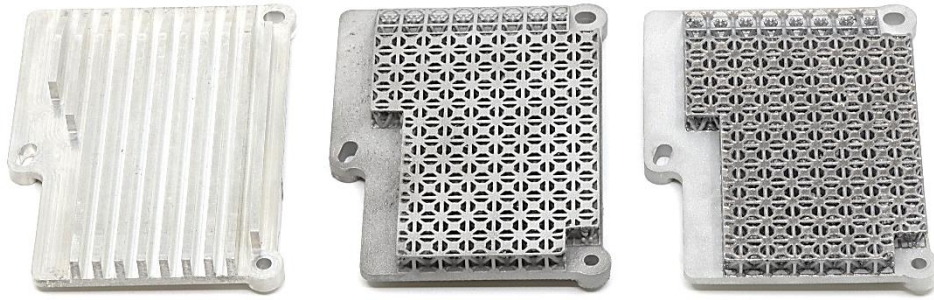
Figure 3-47. Conventional heat sink produced by machining (left), AM heat sink produced by PBF (middle) and HM heat sink produced by machining and PBF (right).
