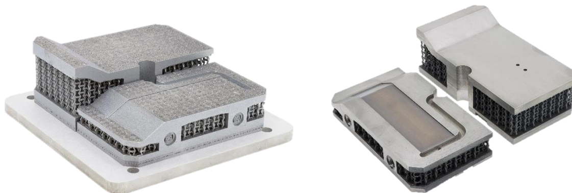
Figure 4-29. Injection moulding inserts produced by additive manufacturing before (left) and after (right) surface finishing (via machining).
