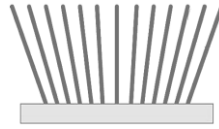
Figure 3-3. Schematics of heat sink with oblique fins (front view) (adapted from [40]).
