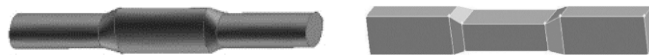
Figure 3-10. Configurations of alternating elliptical channels (left) and alternating rectangular channels (right) (adapted from [70]).
