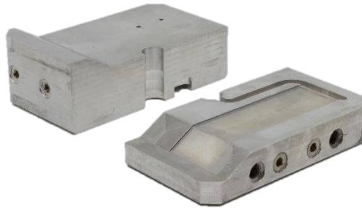
Figure 4-27. Injection moulding inserts produced by subtractive manufacturing with straight-drilled cooling channels.
