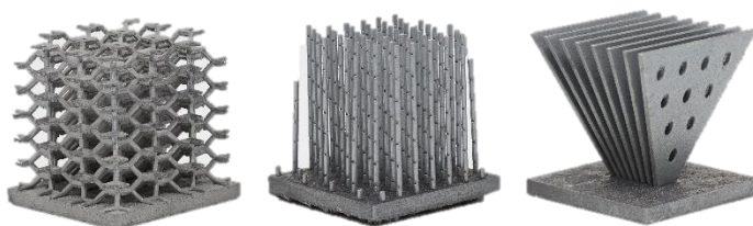
Figure 3-31. Air-cooled heat sinks produced by PBF.
