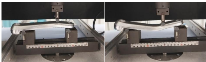
Figure 2-15. Crankset at the beginning (left) and at the end (right) of the three-point flexural test.
