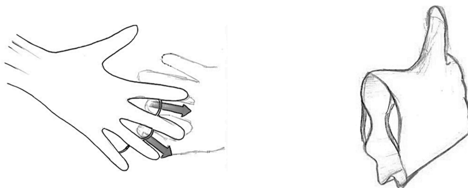
Figure 3. Webbed tabs to help put on and take off the gloves.
