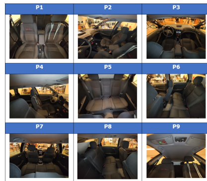
Figure 3: Example of perspectives captured by RGB sensors at positions P1 to P9 inside each car.
