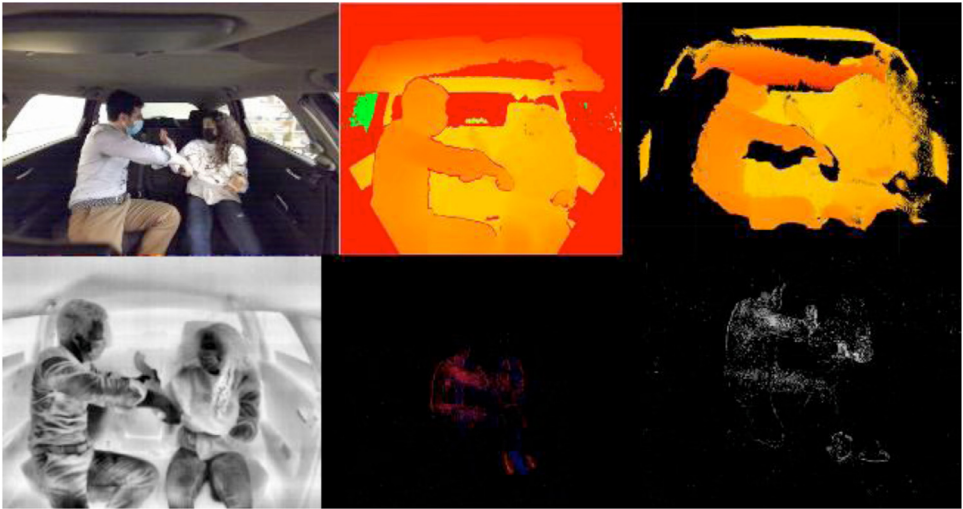
Fig. 4. From Top Left to Bottom Right: RGB, Depth, Point-cloud, Thermal, NVS, and Events Grayscale).
