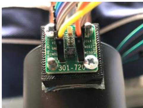
Figure 1: ADXL372 assembled on the riflescope
