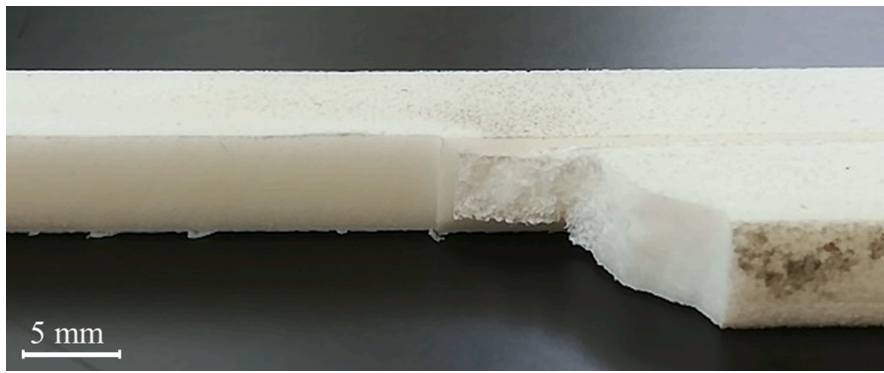
Fig. 4. Representative surface of crack propagation at the end of the DCB test.
