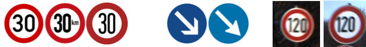
Fig. 2. Sample of intra-class variations per country in GTSRB. Left and middle: variation due to new templates being introduced; Right: variation due to manufacturing.
