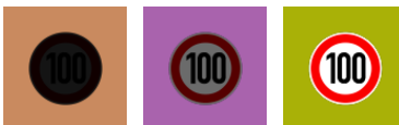
Fig. 8. Brightness variation in synthetic samples of class 7 for the GTSRB dataset. Source [10].
