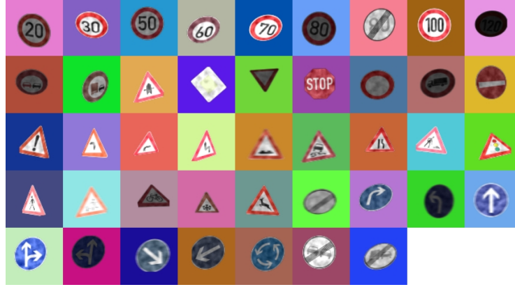
Fig. 13. Samples of generated synthetic traffic signs with solid colour backgrounds for each class of the GTSRB dataset. Source [10].
