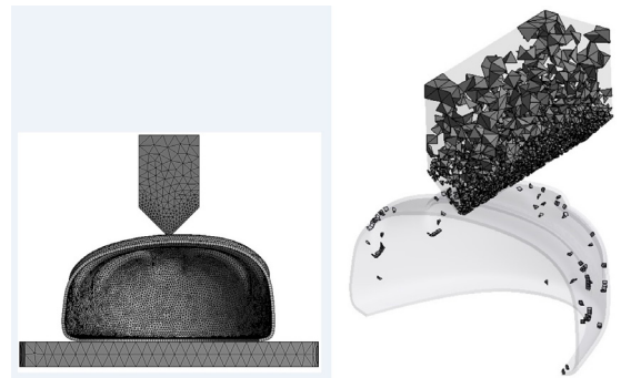
Figure 3. Finite Element model with mesh preview of S3F3 – 1.2 mm.
