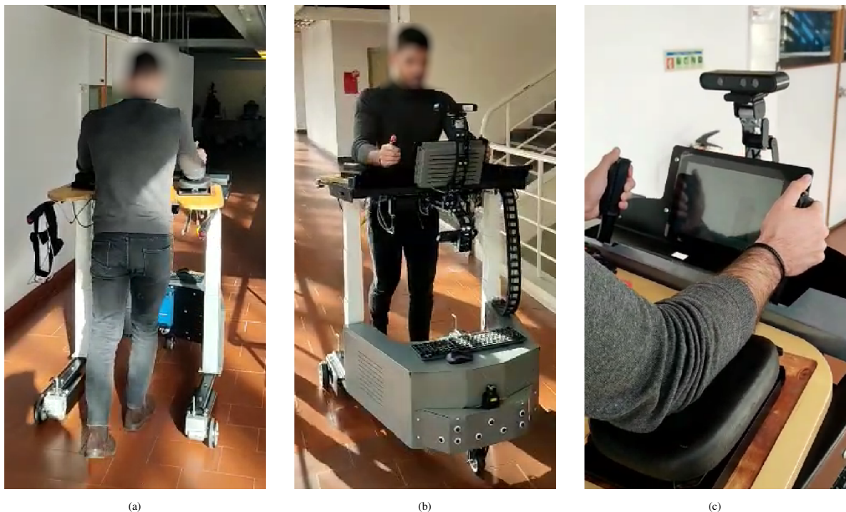
Figure 43: Cognitive Game validation: (a) and (b) Driving the walker, while playing the Cognitive Game; (c) Close up of arms while driving and controlling the walker.
