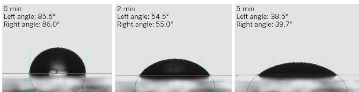
Figure 5.8 – Example of the decreasing contact angle of the rhamnolipids (5 x CMC) produced by Burkholderia thailandensis E264 in CSL medium on an oil-coated glass surface, showing a wettability alteration from oil/neutral-wet (at 0 min) to water-wet (at 5 min).
