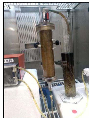
Biosurfactant flooding ( ex situ )
