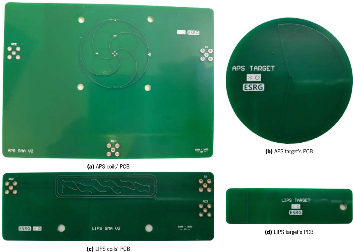
Figure 5.2: Manufactured inductive position sensors' PCB featuring the optimized geometries
