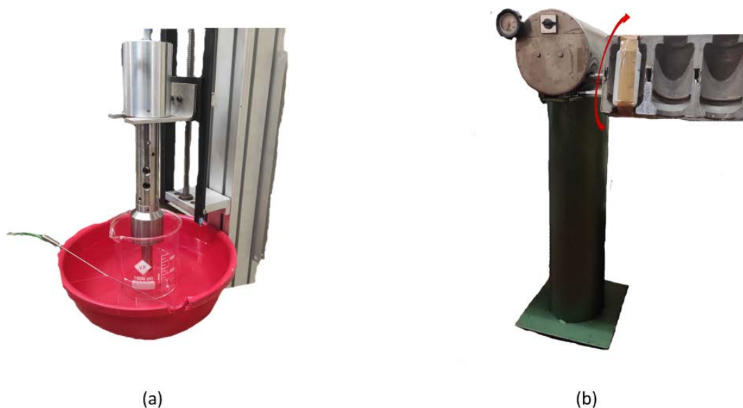
Figure 4.28: Equipment used for the adsorption tests. (a) Ultrasound with the beaker with the solution to treat. The beaker is in a water cooling system with a tank with water. (b) Rotational machine for the mechanical action.
