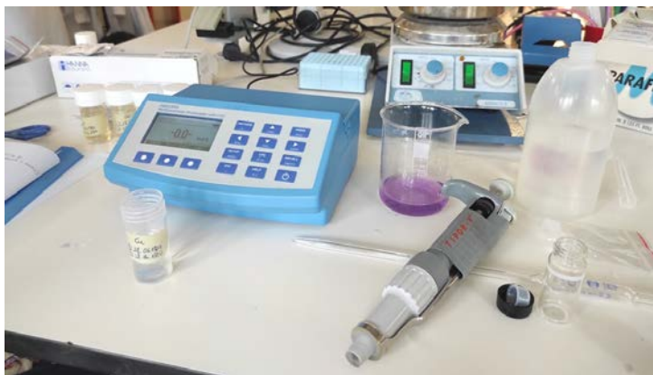
Figure 4.30: Hanna 83300 for the measurement of inorganic pollutants concentration on the samples.
