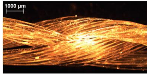
Figure 19 – Optical microscopy picture of the ligament tissue engineering scaffold (127). Reproduced by permission of The Royal Society of Chemistry.
