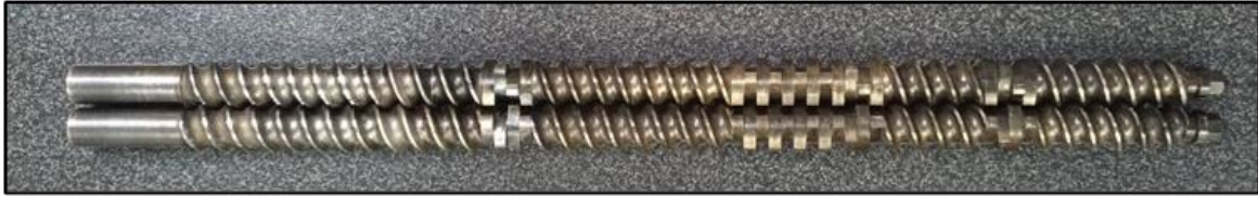
Figure 34 – Screw profile used for the production of the composite filaments. The screws comprise three mixing zones separated by conveying elements. Polymer and fillers are fed at the conveying zone upstream. The polymer melts at the first mixing section. The remaining two mixing zones promote dispersive and distributive mixing.
