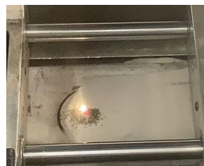
(c) Printing bed: Laser actuation
