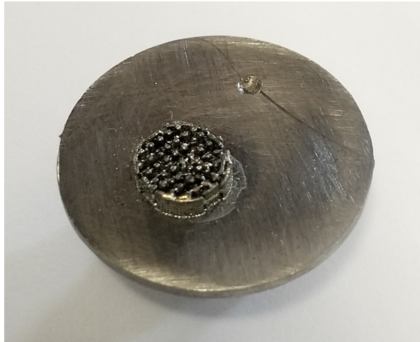
Figure 111: Nd-YAG laser – bi-material manufacturing test: Produced part
