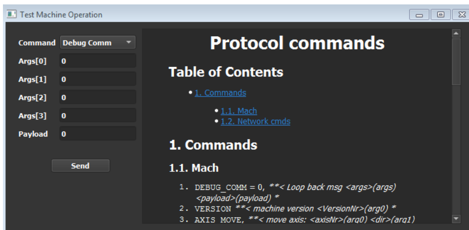
Figure 96: Manufacturing tests: machine's testing dialog
