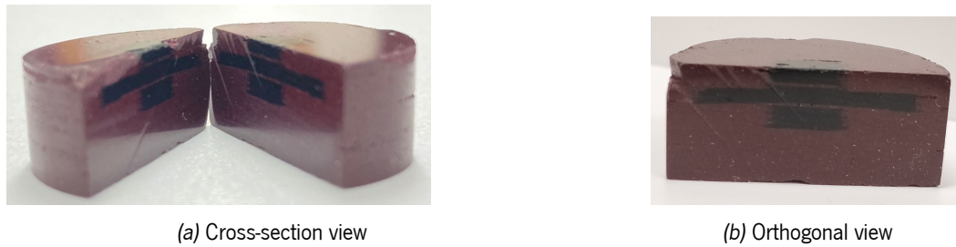
Figure 102: CO 2 laser – bi-material manufacturing test: Produced part
