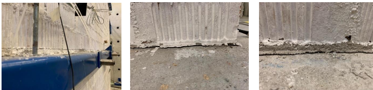
Figure 21 Uplift at the base of the URM walls at Cycle 15 (Base shear force is equal to 75% of the total weight)
