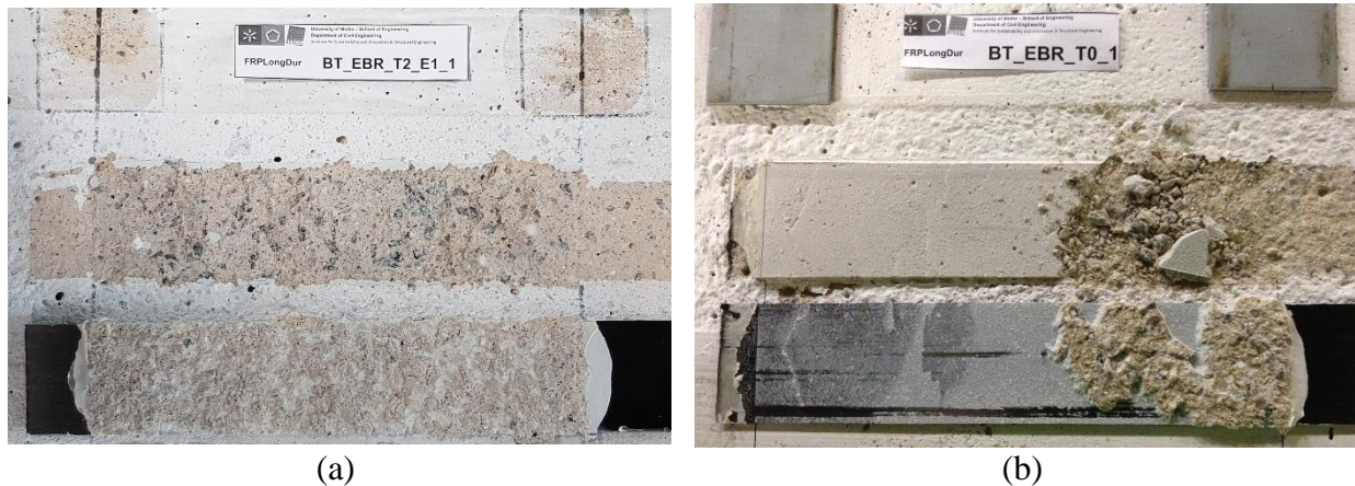
Fig. 9. Failure modes observed in the pull-out shear bond EBR tests: (a) C – cohesive failure of concrete and (b) C + F/A - cohesive failure of concrete and debonding at laminate-adhesive interface.
