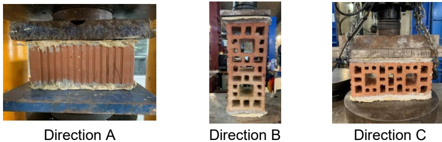
Fig. 2 - Compression test on brick units in different directions
