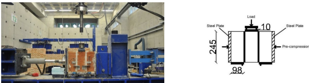
Fig. 11 - Configuration of the test setup for initial shear test and the details of the specimen (in mm)
