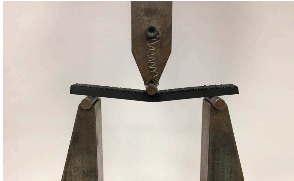
Figure 5. Experimental setup of TPB test.
