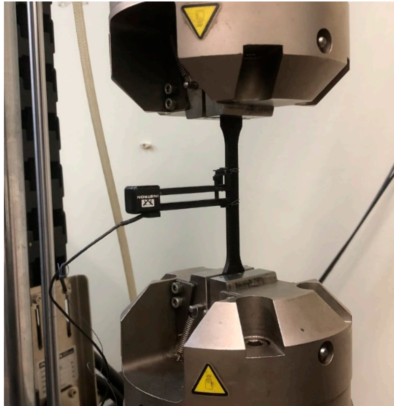
Figure 6. Experimental setup of standard tensile tests.
