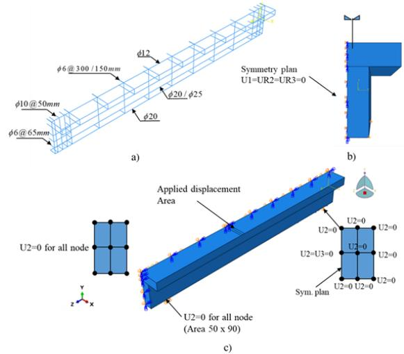
**Figure 7:** Boundary and support conditions.
