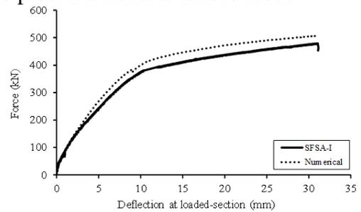
**Figure 13:** Experimental and numerical relationships of force versus deflection of SFSA-I beam.
