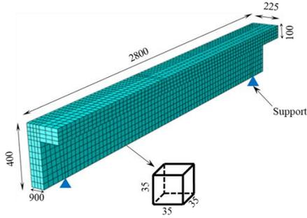
Figure 9: Mesh size of the reference beam (35 mm).
