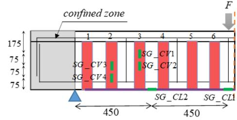
**Figure 3:** Disposition of the strain gauges in the NSM laminates (SG-CL1 and SG-CL2) and EBR U-CFRP (SG\_CV1, SG\_CV2, SG\_CV3 and SG\_CV4) of SFS-I and SFSA-I beams (dimensions in mm) [5].
