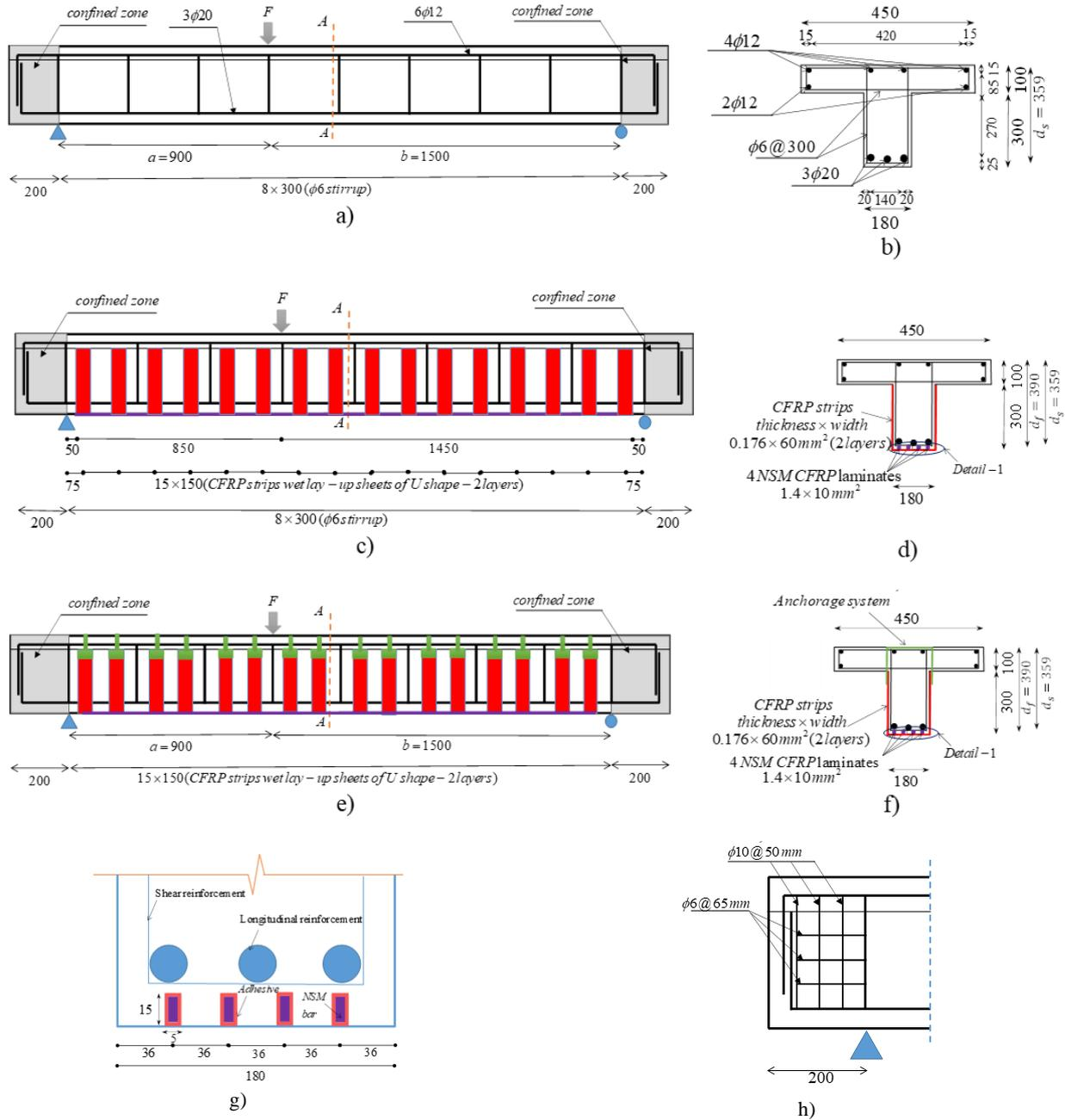
**Figure 1:** Series I of the experimental test [5] (dimensions in mm): a) reference beam (REF-I), b) section A-A of REF-I, c) strengthened beam without anchorages (SFS-I), d) section A-A of SFS-I, e) strengthened beam with anchorages (SFSA-I), f) section A-A of SFSA-I, g) detail-1, h) confined zone detail.
