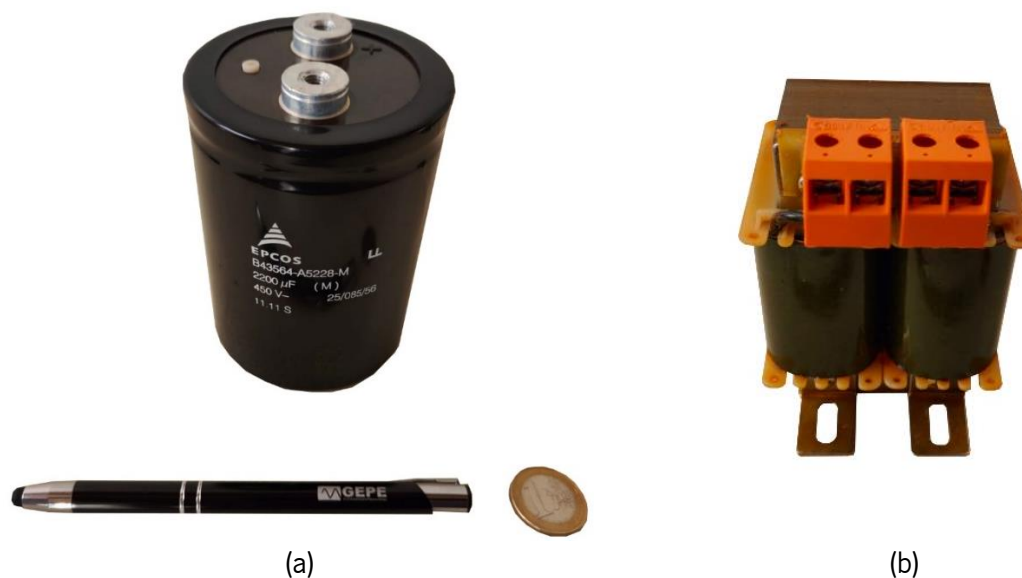
Figure 5.22 Passive elements in the power circuit: (a) decoupling capacitors; (b) coupling coils.
