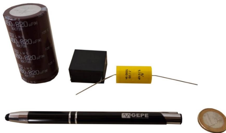
Figure 5.2 Capacitors selected for the submodule development, 450 V 820 \mu\text{F} , 500 V 10 \mu\text{F} , 1000 V 100 nF, respectively.
