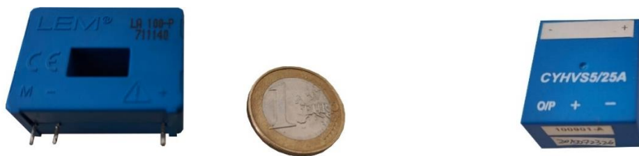
Figure 5.3 Sensors equipped in the submodules: Current sensor and Voltage sensor.
