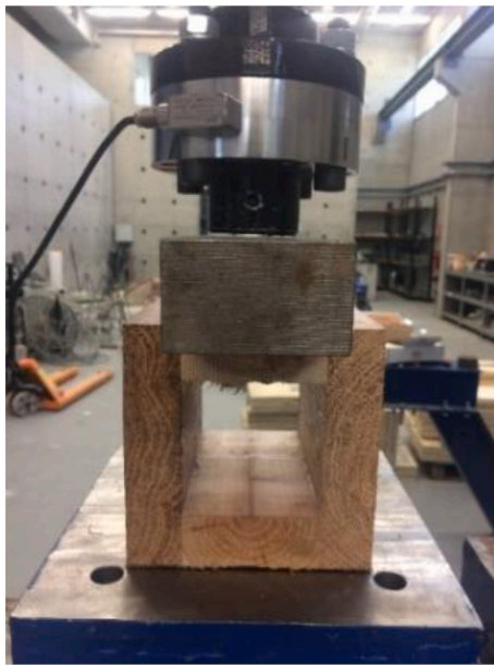
Fig. 6. Test setup for the load applied on the upper wooden element.
