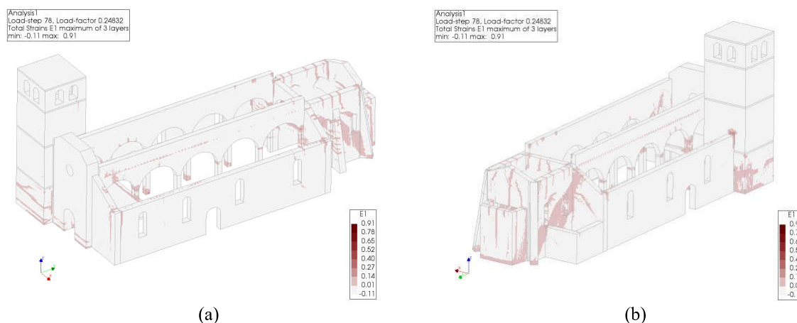
Figure 10: Maximum principal strains E1, y-direction (a) front view; (b) rear view
