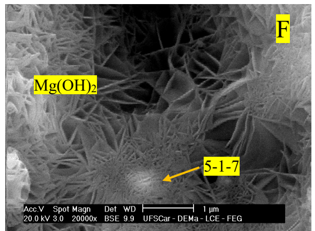
Figure 3: Scanning electron microscopy (SEM) images of carbonated and non-carbonated MOS-based fiber cement boards. (A), (B), and (D) represent the non-carbonated reference samples (Ref); (C) Carb24; (E) Carb72 and (F) Carb48.
