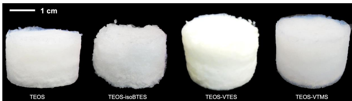
Figure A5. Appearance of the polyester-reinforced aerogel composites, developed with different co-precursors (the silica system used is described under each image), with the same mass of polyester fibres, and keeping the volume of the precursor and co-precursor constant.
