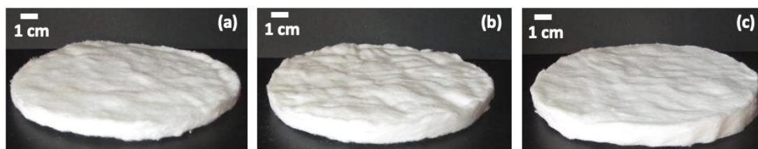
Figure 5. Scaled-up cotton-reinforced silica aerogel composites, custom-built for sound adsorption analyses: (a) conventional cotton mat with \sim 8.5\text{ wt}\% of fibres; (b) conventional cotton mat with \sim 13.5\text{ wt}\% of fibres; (c) compressed cotton mat with \sim 12.4\text{ wt}\% of fibres.
