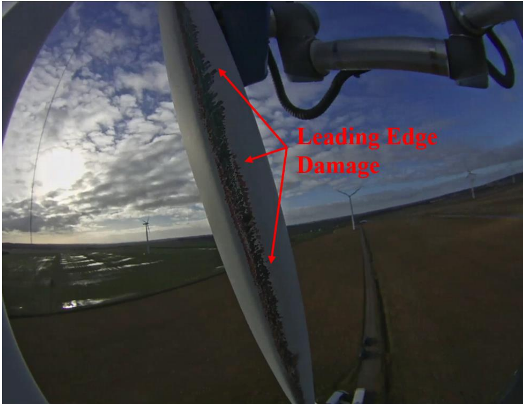
Figure 2.10: Leading edge erosion of a WTB detectable via visual inspection. Source [29]
