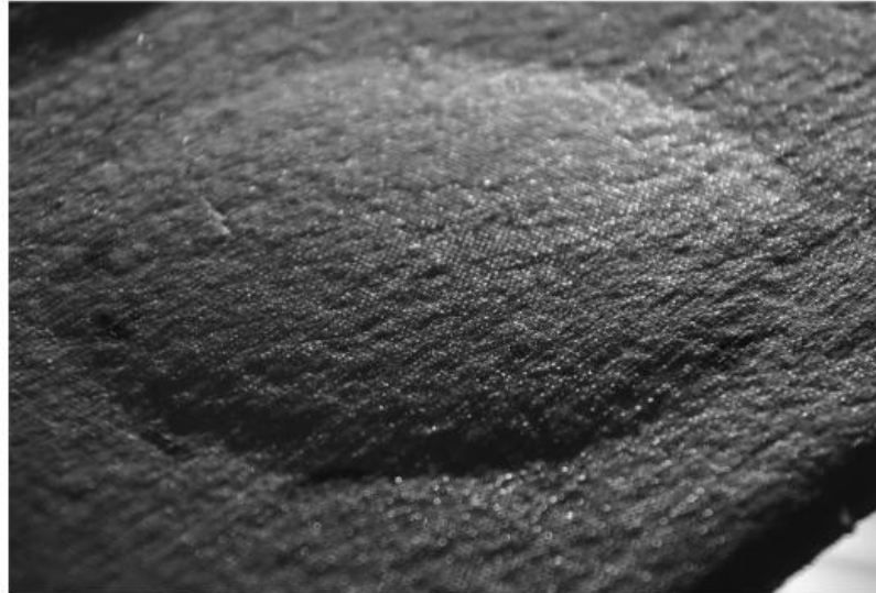
Figure 2.9: Blistering on the surface of a composite material. Source [28]
