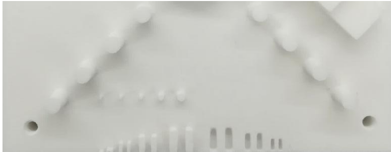
Figure 3.74 Fine features of a test artefact produced by SLS with 0.007 J/mm ( P_{\text{Laser}}/S_{\text{Speed}} ).
