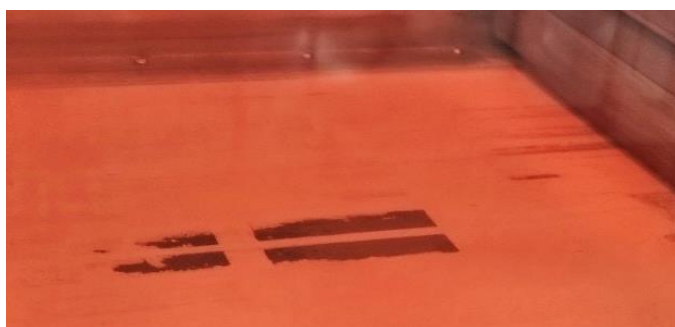
Figure 4.42 Sintering process of PA12-GNP composites evidencing difficulties in powder spread.
