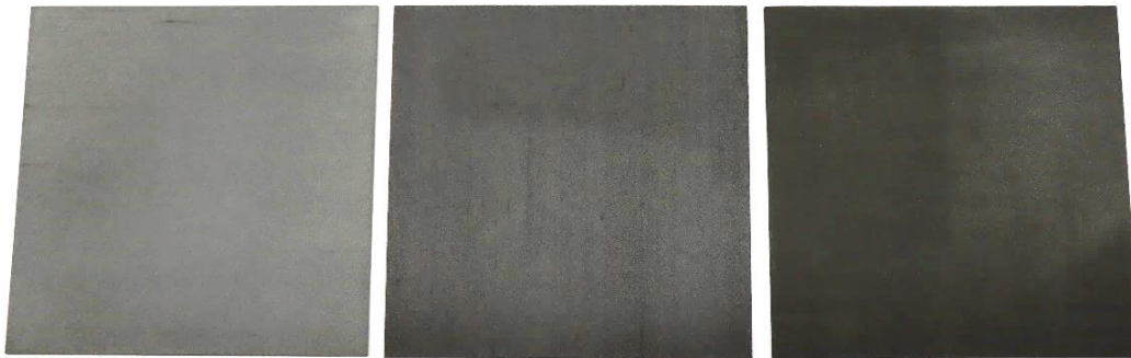
Figure 4.44 Surface finishing of test specimens produced by SLS with PA12 incorporating 0.50 wt% (left), 1.75 wt% (middle) and 3.00 wt% (right) of GNP.
