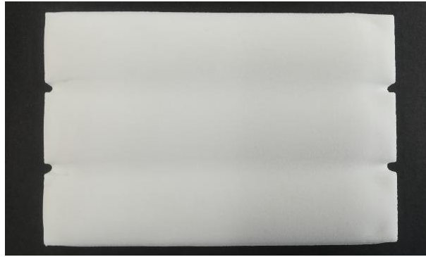
Figure 3.22 Test specimens produced by SLS with 0.318 J/mm 3 in the xy-direction-simultaneous.
