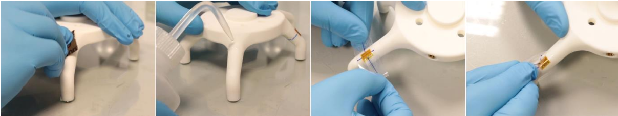
Figure 5.10 Installation of the strain gauges in a PA12 prototype.
