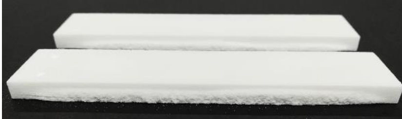
Figure 3.14 Lateral defects in test specimens produced by SLS with 0.358 \text{ J/mm}^3 .
