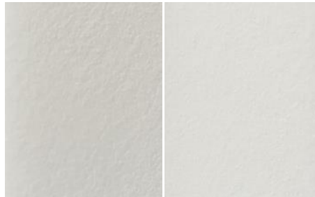
Figure 3.10 Finishing of surfaces directed to the top (left) and bottom (right) of test specimens produced by SLS with 0.198 J/mm 3 .
