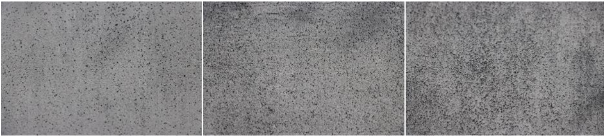
Figure 4.10 Top surface of test specimens produced by SLS with PA12 incorporating 0.50 wt% (left), 1.75 wt% (middle) and 3.00 wt% (right) of MWCNT.
