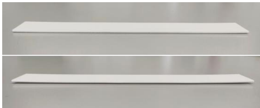
Figure 3.99 Test bars produced by SLS with single (top) and multiple (bottom) exposure types.
