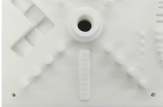
Figure 3.17 Surface of a test artefact produced by SLS with 0.318 \text{ J/mm}^3 in the x-direction after cleaning with sand blasting.
