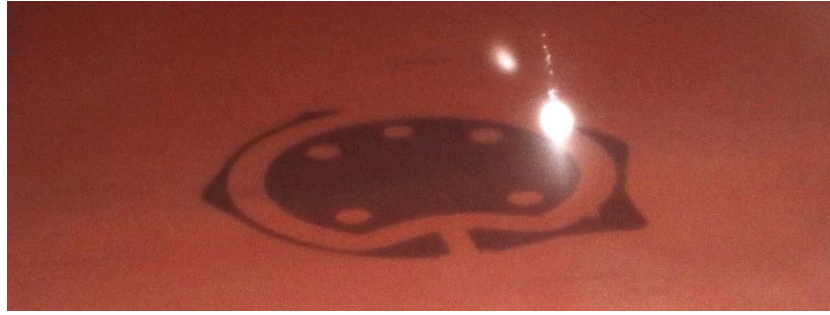
Figure 5.8 Production of a PA12-GNP prototype by SLS.
