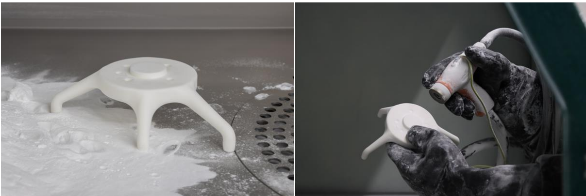
Figure 5.7 Prototype produced by SLS with PA12.
