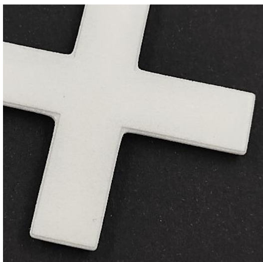
Figure 3.95 Details of a test specimen produced by SLS with combination of parameters (30% of t_{Skin}/t_{Part} ).
