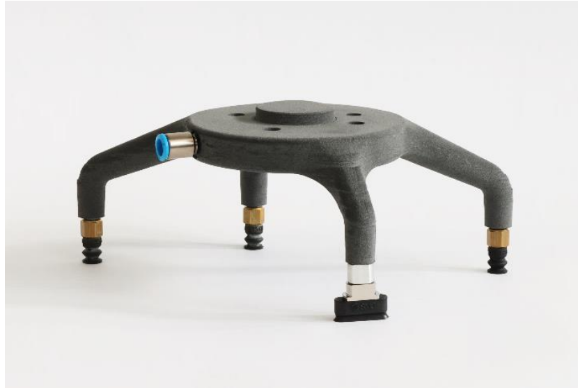
Figure 5.38 Robot end-effector produced with PA12-GNP (final version).
