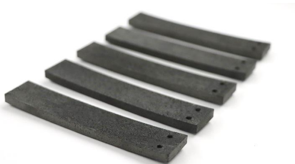
Figure 4.11 Warpage in test specimens produced by SLS with PA12 incorporating 3.00 wt% of MWCNT.
