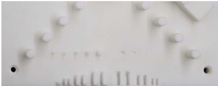
Figure 3.92 Fine features of a test artefact produced by SLS with combination of parameters (20% of t_{\text{Skin}}/t_{\text{Part}} ).
