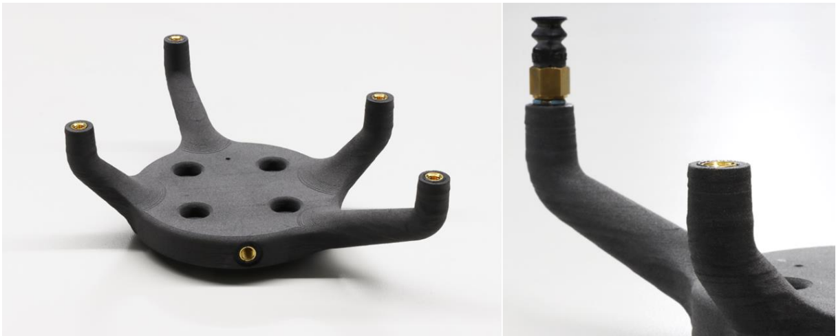
Figure 5.9 Prototype produced with PA12-GNP evidencing metallic inserts.
