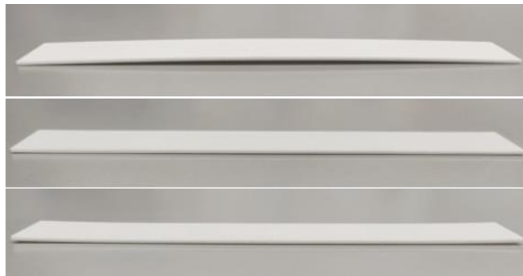
Figure 3.23 Test bars produced by SLS with 0.158 J/mm 3 (top), 0.278 J/mm 3 (middle) and 0.398 J/mm 3 (bottom).
