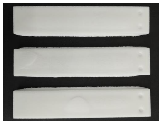
Figure 3.16 Lateral defects in test specimens produced by SLS with 0.398 \text{ J/mm}^3 .
