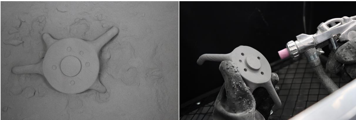
Figure 5.6 Prototype produced by SLS with PA12-GNP.
