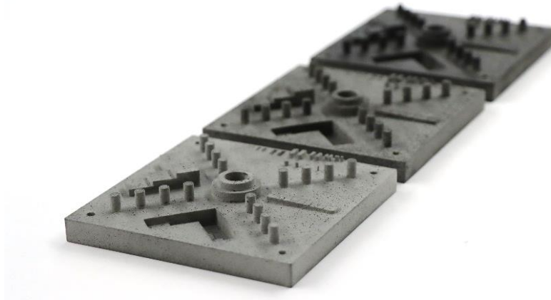
Figure 4.9 Test artefacts produced by SLS with PA12 incorporating 0.50 wt%, 1.75 wt% and 3.00 wt% of MWCNT.
