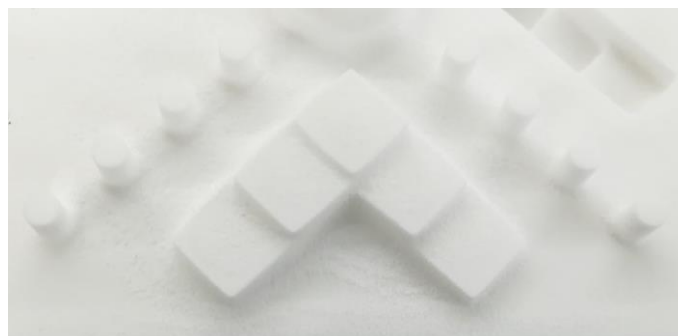
Figure 3.13 Surface of a test artefact produced by SLS with 0.358 \text{ J/mm}^3 after cleaning with microbeads blasting.
