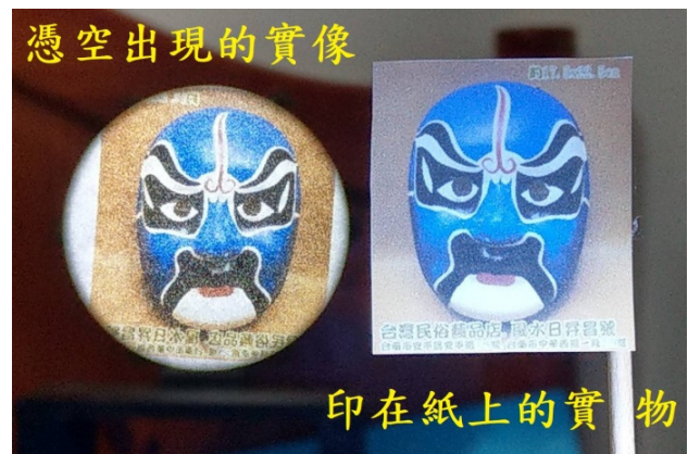
Figure 14. The real image can be observed directly, just like a real object (left)
