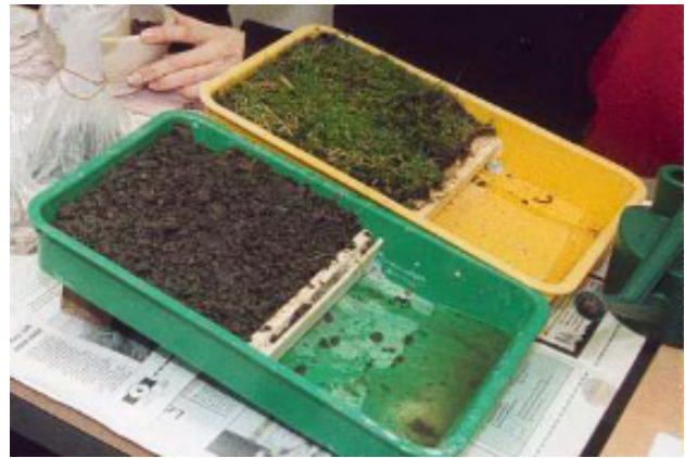
Figure 4. Set up for percolation practical [2]
