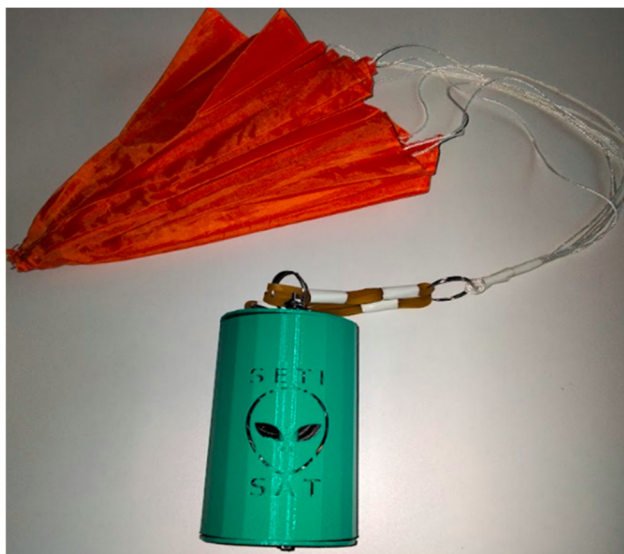
Figure 14. Final appearance of the transmitter with parachute.
