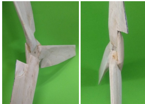
Figure 13. Carving, planing, and sanding wooden blades for assembly into a three-blade wind turbine. Increasing the root section thickness before machining enables a significantly larger installation angle in that area
