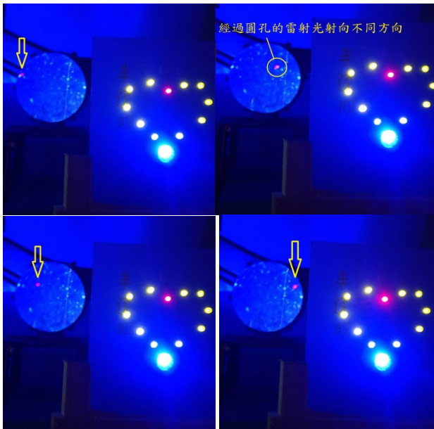
Figure 12. The laser beam hits different portions of the concave mirror but is consistently reflected to the same point
