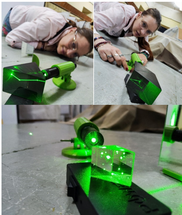
Figure 8. Visualisation of light rays' trajectory through one and several prisms
