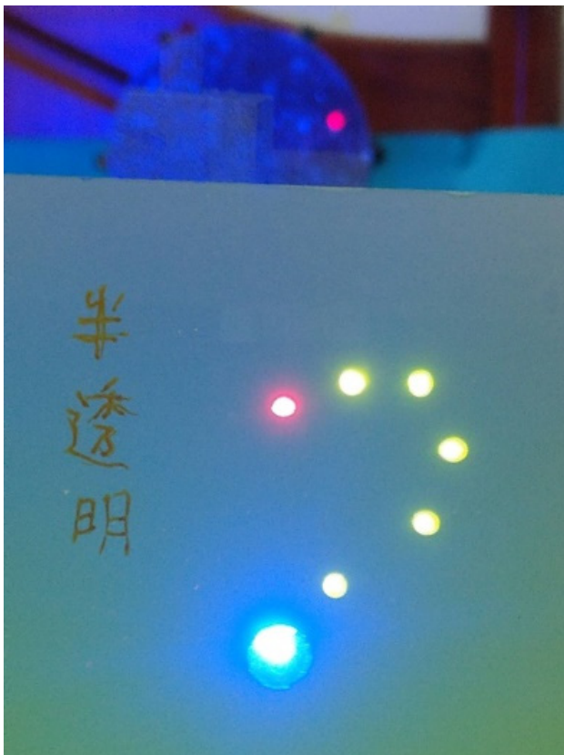
Figure 13. We sequentially light up the other LEDs to emphasize the object or a real image consists of numerous point source of light
