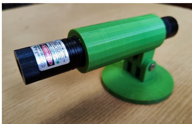
Figure 3. Laser pointer, installed into a holder made by 3D printing
