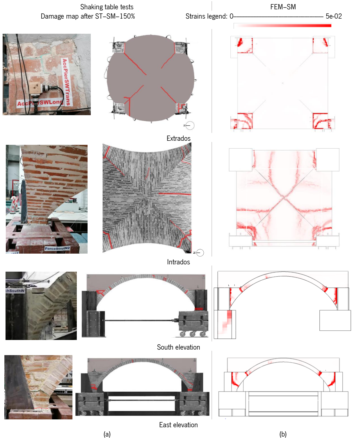
Figure 7-19. Damage map for: (a) ST-SM-150%, (b) principal strains distribution in FEM-SM model.
