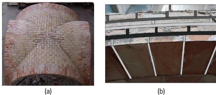
Figure 2-10. Torres et al. (2019)'s specimen: (a) timbered vault model, (b) detail of the thickness section.
