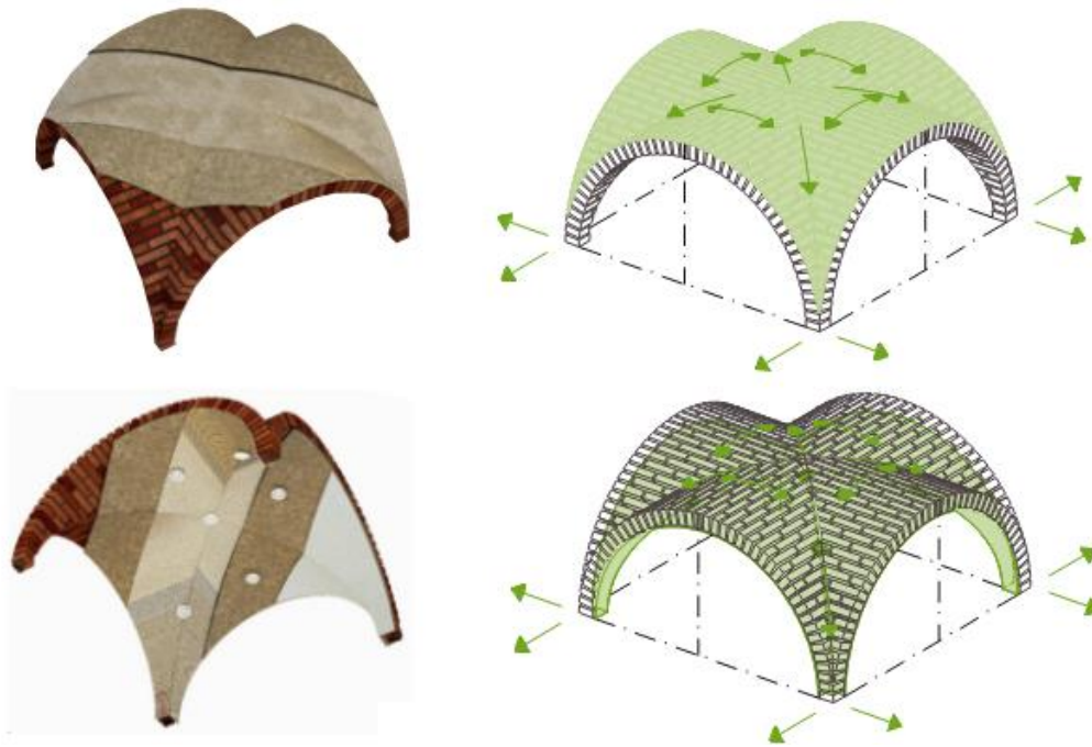
Figure 1-19. Extrados and intrados disposition of TRM on masonry cross vault (Kerakoll guidelines).
