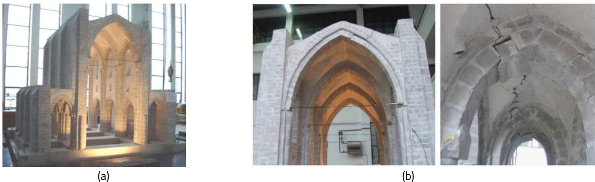
Figure 2-4. De Matteis et al. (2010)'s experimental campaign: (a) illustration of the positioning on the shaking table, (b) photographs of the details of the main damage.
