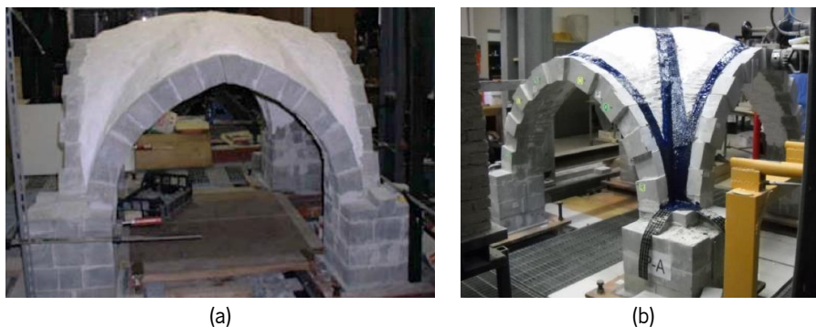
Figure 2-6. Fagone et al. (2016)'s experimental campaign: (a) unstrengthened specimen, (b) strengthened specimen with CFRP continuous sheet at the extrados.
