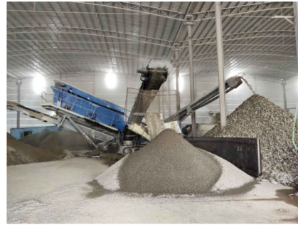
(b) Crushing of precast rejects in the workshop
