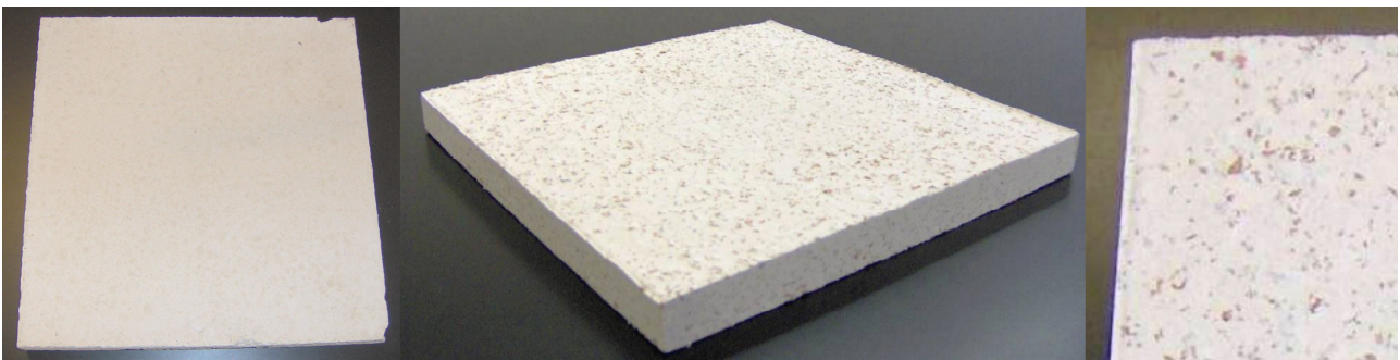
Fig. 6 - Board of pressed gypsum Fig. 7 and Fig. 8 - board of pressed gypsum with paper and cork and texture
